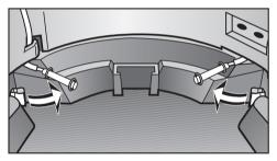
■ Loosen the water sensors and carefully bend them upwards.
